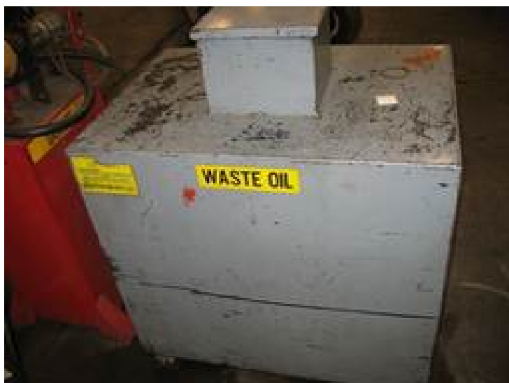
Used oil tank incorrectly labeled as “Waste Oil.”
